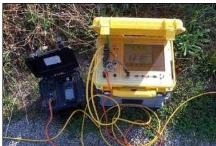
FIG. 09 – SISMOGRAFO UTILIZZATO MAE A6000S.
