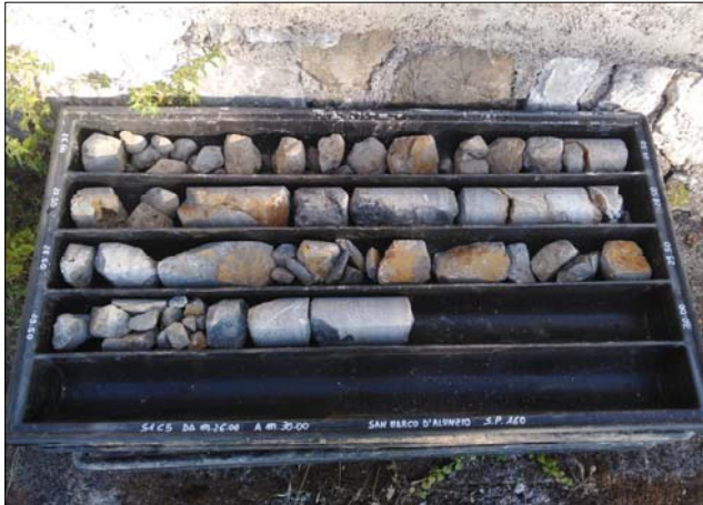
Foto 6: Sondaggio S1 - Cassetta 5 da 26,0 a 30,0 mt
